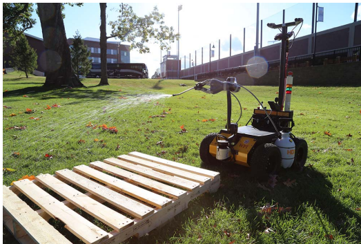
Fig. 4. A teleoperated robot demonstrating a decontamination operation. Many tasks that do not involve contact with patients such as logistics, materials handling, and decontamination can be accomplished using teleoperated or semiautonomous robots to enhance the safety of workers.
