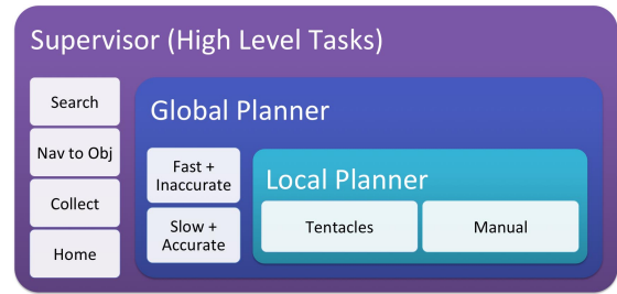
Figure 5. The three levels of the hierarchical control. The supervisor coordinates the mission-level tasks. The global planner plans beyond the sensor horizon on the global map. The local planner plans on a local map representing a snapshot of the current environment around the robot.
