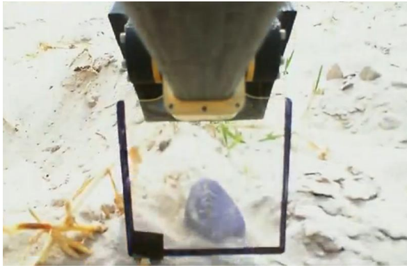
Figure 4. ORYX 2.0 picking up a purple sample rock in JSC sand pit. The clear polycarbonate plate and small piece of tape in the corner proved very effective in lining up the manipulator to conduct a pickup operation.
