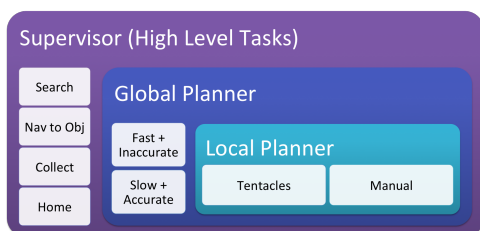
Fig. 2. The three levels of the hierarchical control. The supervisor coordinates the mission-level tasks. The global planner plans beyond the sensor horizon on the global map. The local planner plans on a local map representing a snapshot of the current environment around the robot.
